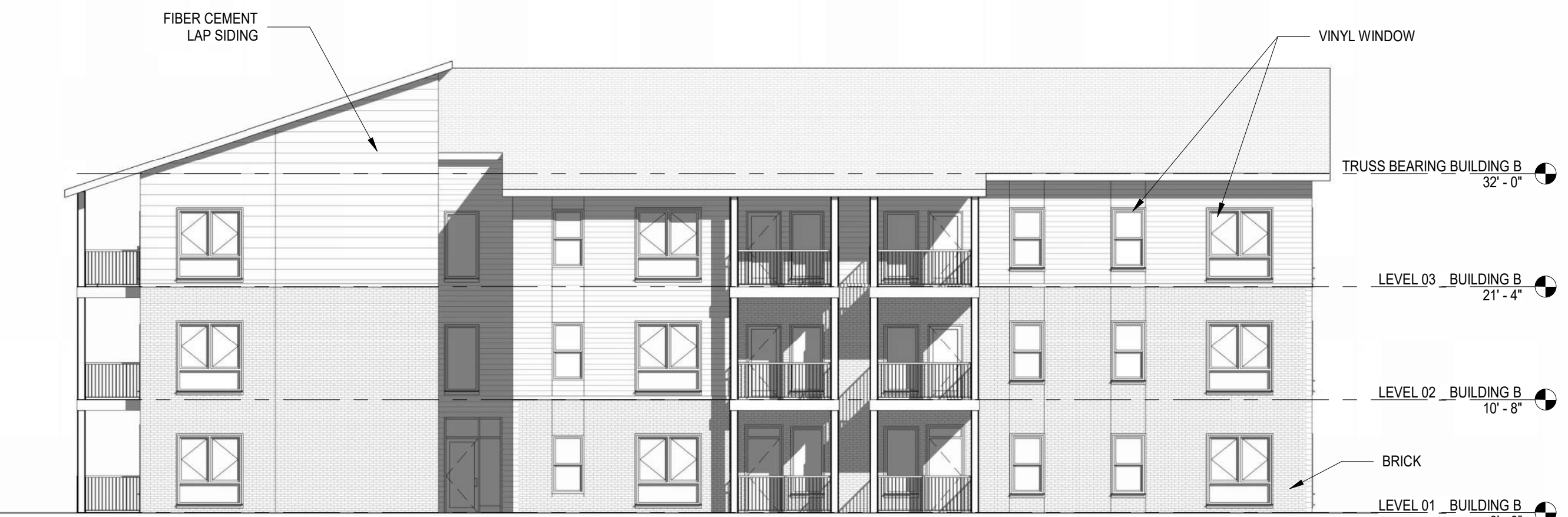
3 WEST ELEVATION BUILDING B A03 3/32" = 1'-0"
