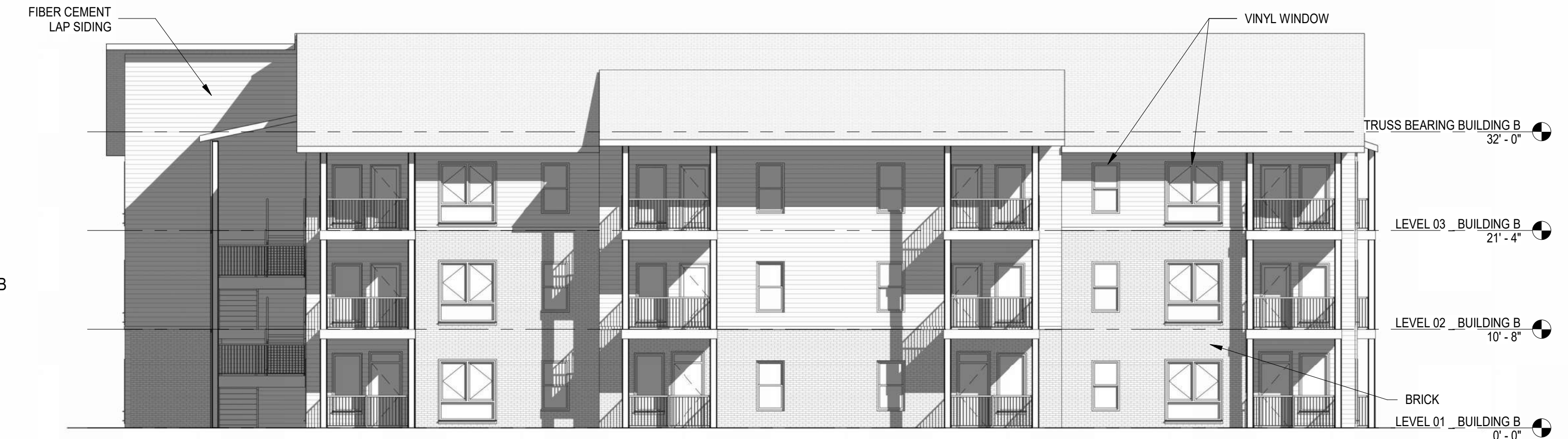
1 NORTH ELEVATION BUILDING B A03 3/32" = 1'-0"
