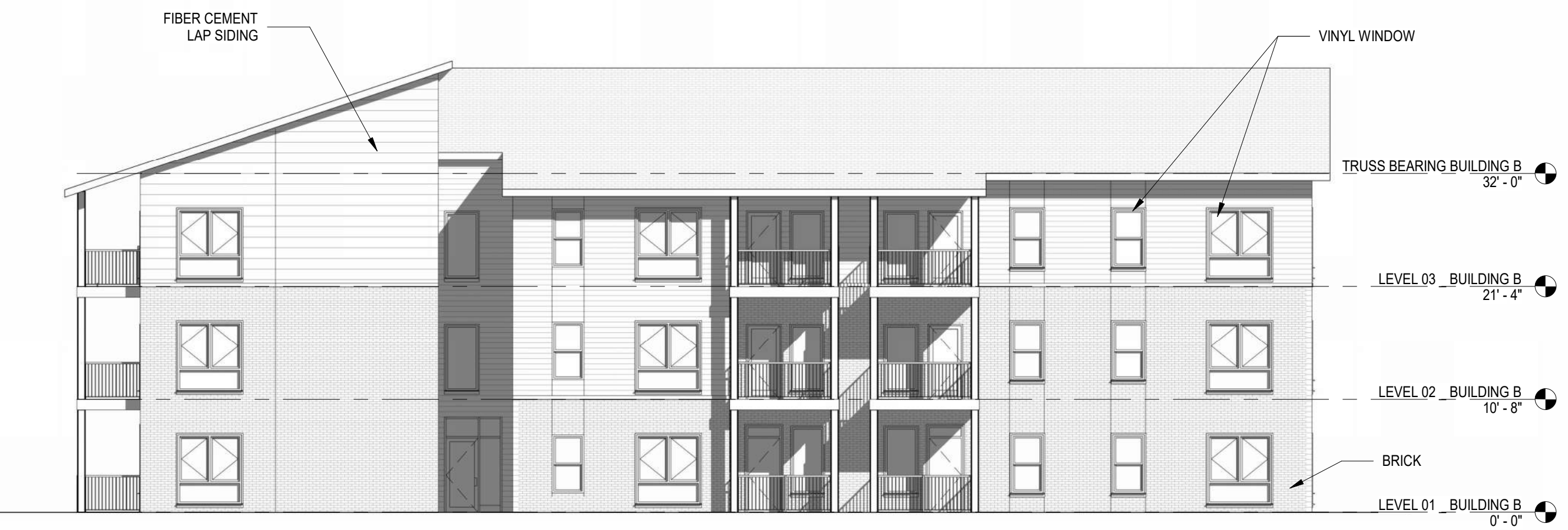
3 WEST ELEVATION BUILDING B A03 3/32" = 1'-0"
