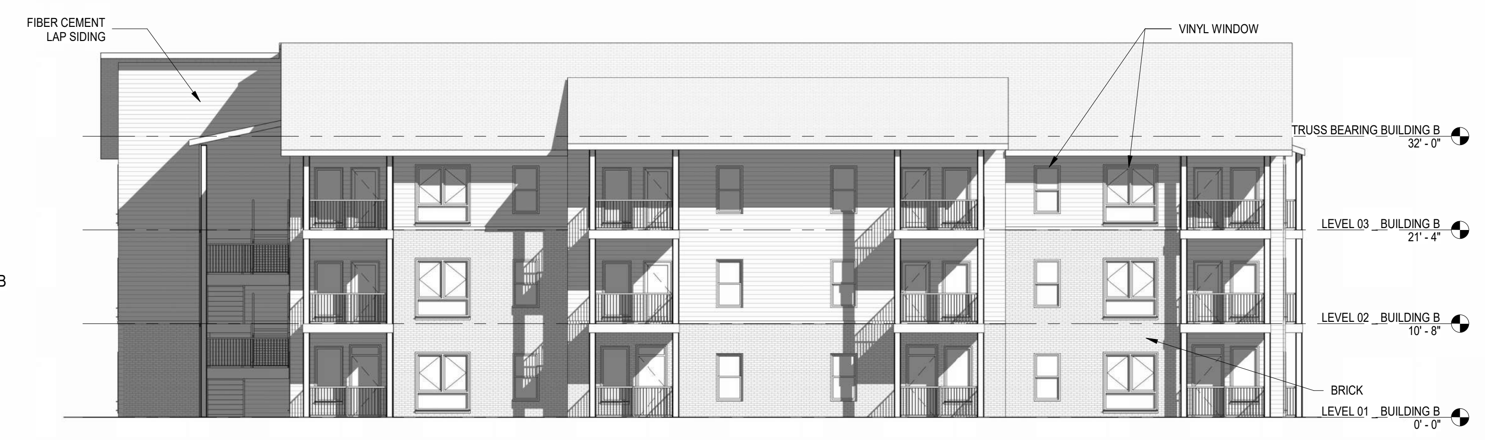
1 NORTH ELEVATION BUILDING B A03 3/32" = 1'-0"
