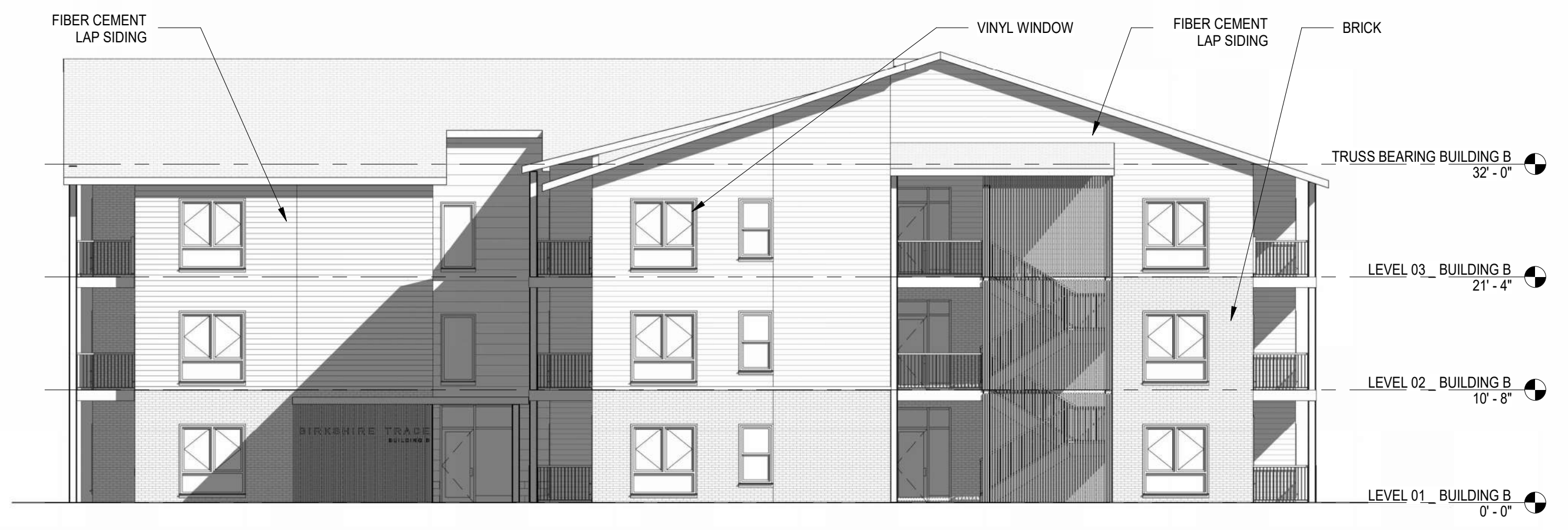
2 EAST ELEVATION BUILDING B A03 3/32" = 1'-0"
