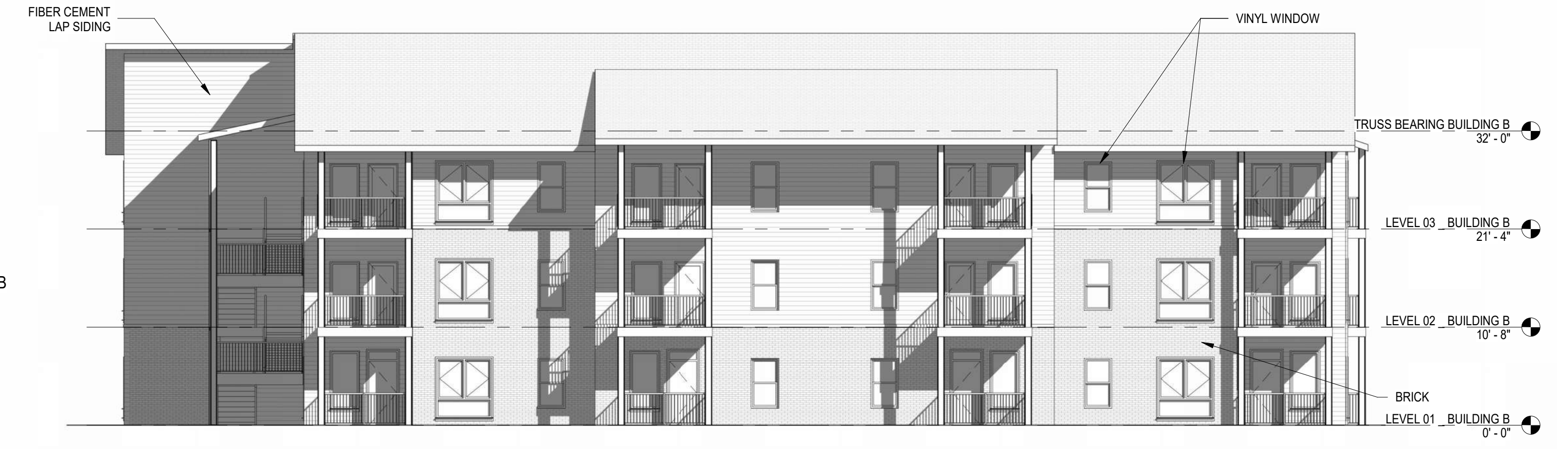
1 NORTH ELEVATION BUILDING B A03 3/32" = 1'-0"
