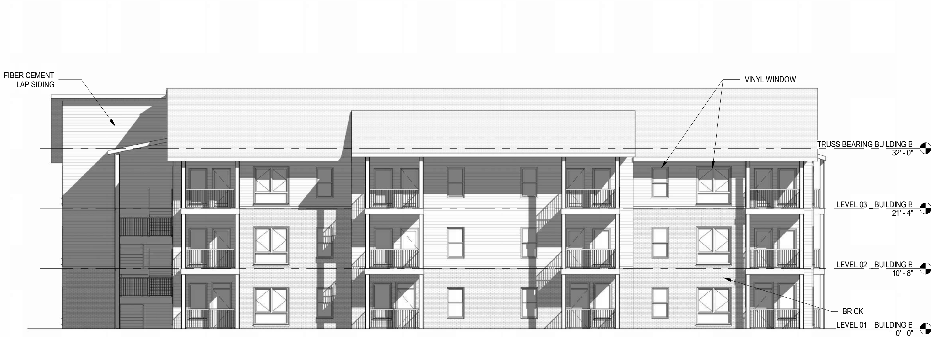
1 NORTH ELEVATION BUILDING B A03 3/32" = 1'-0"
