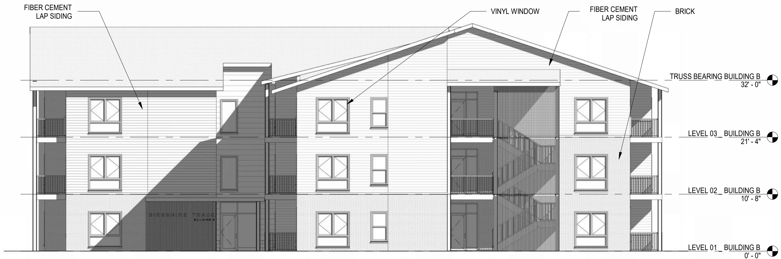
2 EAST ELEVATION BUILDING B A03 3/32" = 1'-0"
